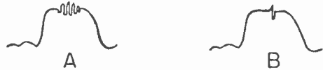
Figure 13. A pattern like that shown in A will be obtained when the input of a wide-band oscilloscope is used. To obtain a usable trace like that in B the frequency response of the scope must be temporarily decreased by connecting a small condenser across the input or by using a resistive isolating probe.
