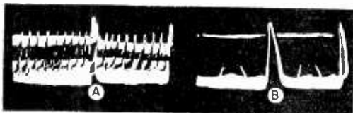
Figure 6. Waveform at the output of the first sync separator stage (V1) with the oscilloscope synced at half the field rate (A), and at half the line rate (B).
