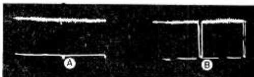
Figure 7. Waveforms at the output of the second sync separator stage (V-2) with the oscilloscope synced at half the vertical rate (A), and at half the horizontal rate (B). Note the almost complete absence of picture information; only the sync pulses remain.
